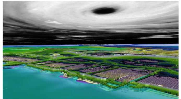
**Figure 3: Rendering of the high-resolution of the terrain elevation model of the city of New Orleans, as obtained by LIDAR measurements, overlaid with ADCIRC surge data and GOES-12 satellite imagery, from [17].**
