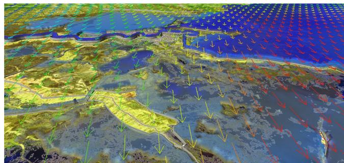
**Figure 2: Detail of the Louisiana coast depicting the hurricane's wind velocities and the surge, as obtained from two different simulations (MM5 vs. ADCIRC).**
